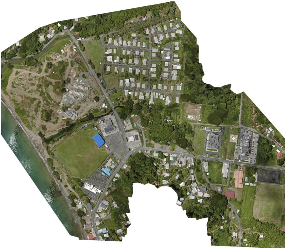
Figure 18. Orthomosaic of Roxborough monitoring site map flown at 120m AGL using DJI Matrice 300 RTK.
